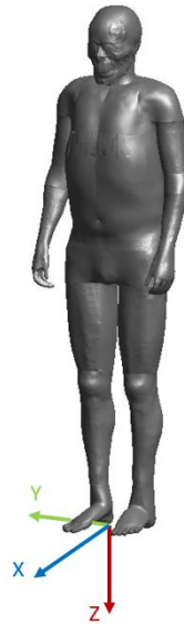
Figure 2: HBM in reference to global coordinate system
